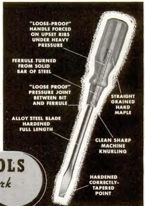
CHARACTERISTICS OF A GOOD SCREWDRIVER
